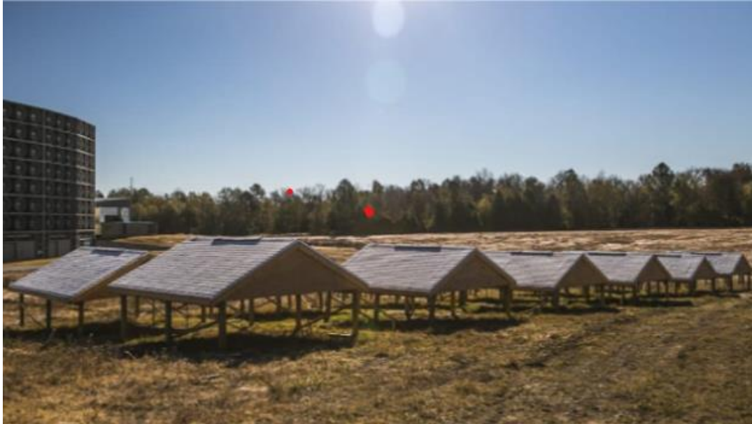
Roof Aging Farm, IBHS Research Center Photo Credit: Insurance Institute for Business and Home Safety
