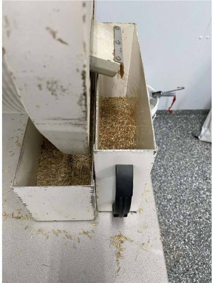
Figure 14. Impact Separator 'in-action' producing in-hull grain for malting
