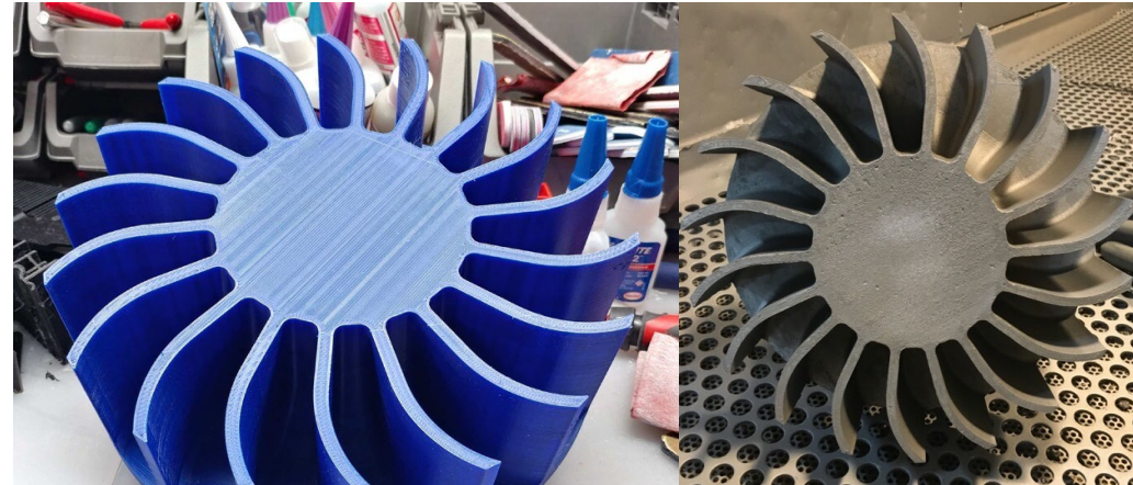
Metal Casting Positive images for molds are accurate, cost-effective, and burn out cleanly with no residues.
