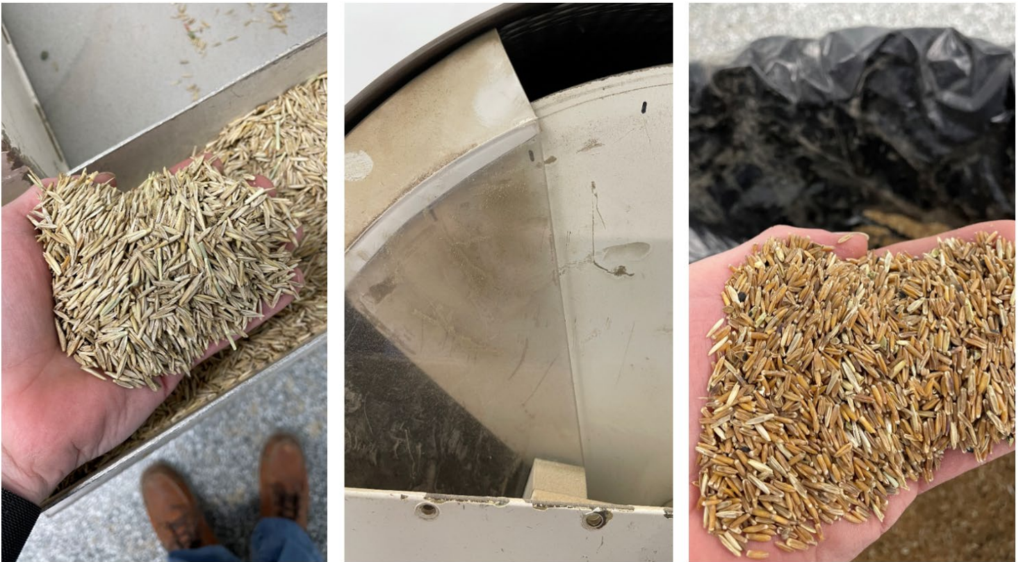
Figure 16. Meyer Color Sorter Adjusted for Cleaning Ergot and Small Black Weed Seeds from Kernza®
