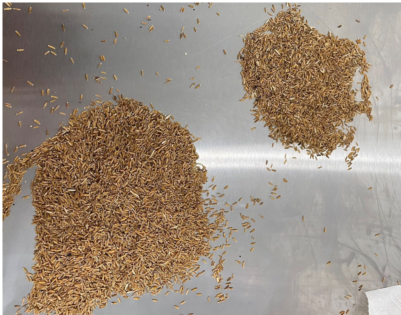
Figure 17. Kernza® before (top right) and after (bottom left) Meyer Color Sorter
