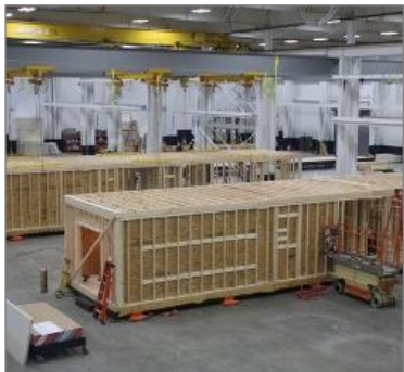
Modular Units are Manufactured Inside Climate Controlled Factory
