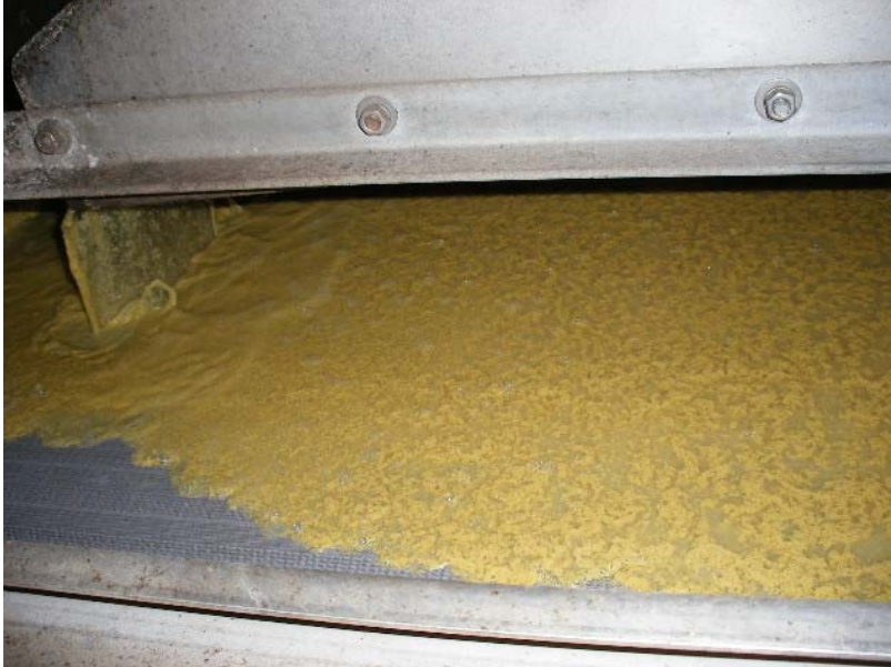
Figure 7 Thin Stillage, Carrier Water and Polymer Mixture on the Belt
