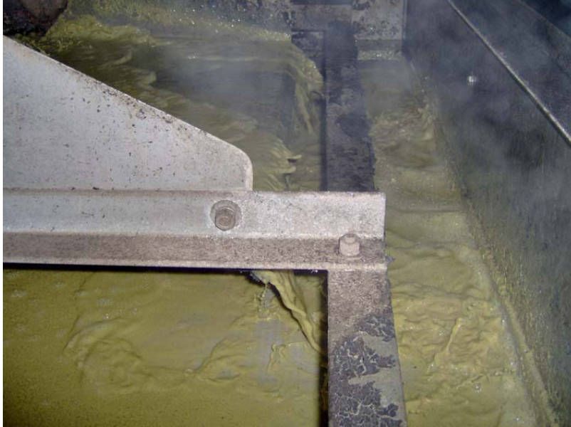
Figure 6 Thin Stillage, Carrier Water and Polymer Going onto Filter
