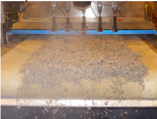
Steam rises from beet pulp exiting the microwave dryer.
