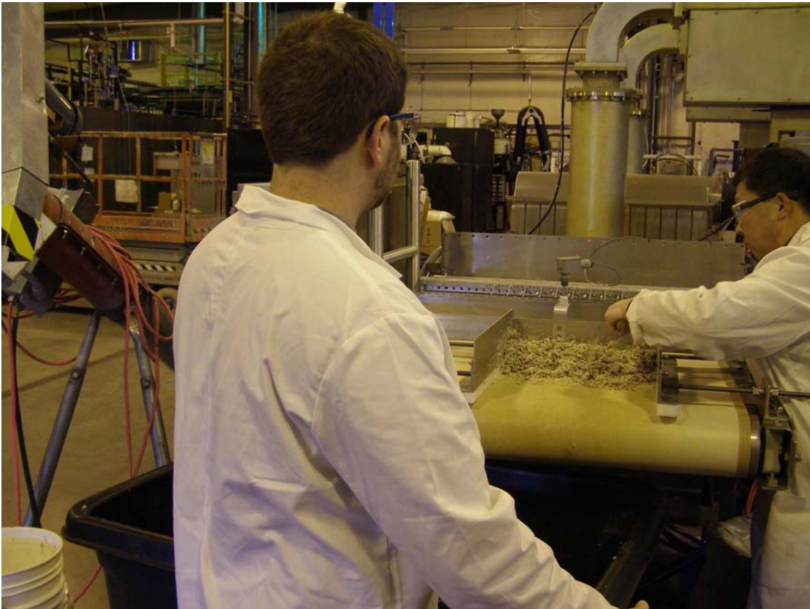
Beet pulp enters the microwave chamber via a conveyor belt. What enters is adjusted for width and height.
