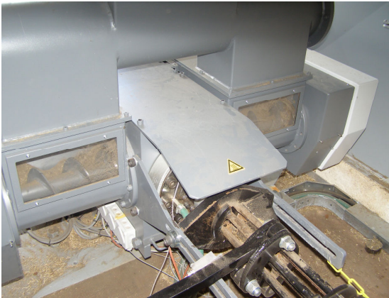
Picture 17: The twin-screw ram briquetter, manufactured by C.F. Nielson, that was located on the site of Pallet Minnesota in Emily, Minnesota.
