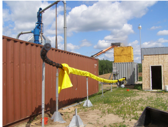
Picture 18: The C.F. Nielson ram briquetter was located in the gray shed to the right, rear. Briquettes travel the entire yellow line into the foreground left. Material that feeds the briquetter enters through the orange conveyor to the rear over the gray shed.
