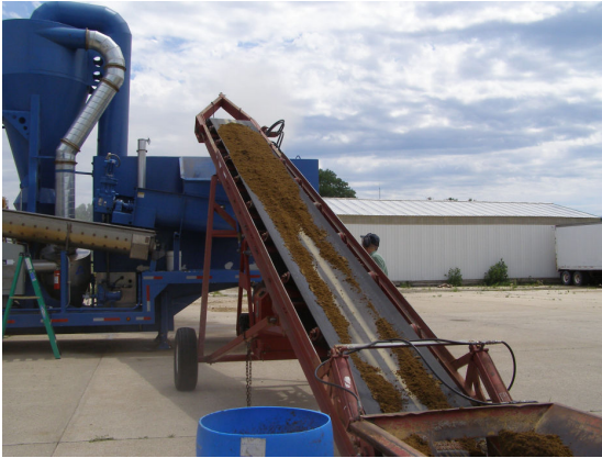
Picture 1: ~65% moisture post-digester solids being fed into Big Blue unit using conveyor
