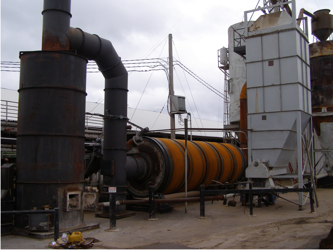
Picture 6: Van der Geest Dairy's installation of a Heil triple-pass rotary drum dryer fueled with ~10% moisture dried manure product. The burning chamber is the upright cylinder to the left; the rotary drum dryer is orange and center; the hopper feeding dried manure is grey and right; upright cyclone and structure to the right/back are part of the processes for storing manure solids to be used for bedding, dried to ~ 20% moisture.
