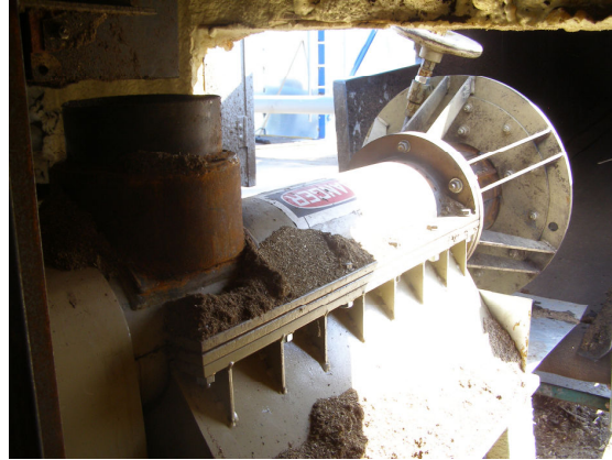
Picture 16: The other side the Rotary Biomass Dryer. On the left is where material feed into the dryer.
