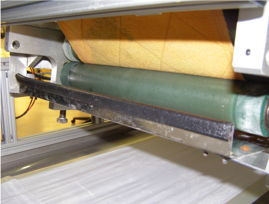
Picture 13: The underside of the former AVS SLS model, where the adsorbent belt (orange) is wrung out after wicking water from the bottom of the filter belt.
