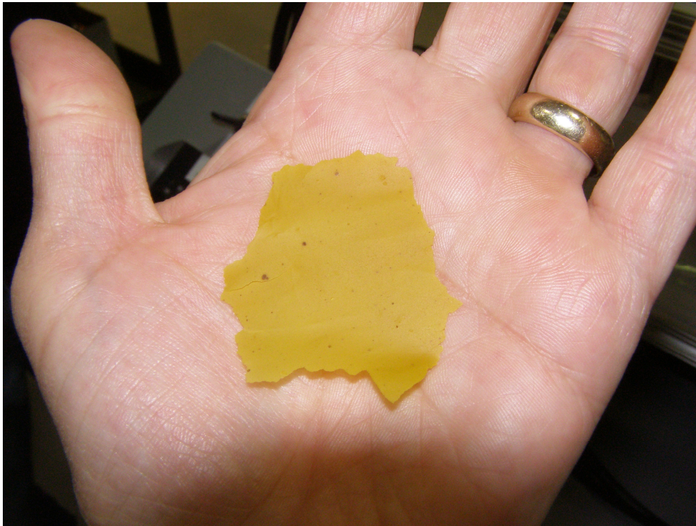
Picture 14: Dried ethanol soluble with bright yellow color fail to show darken color associated with scorching.
