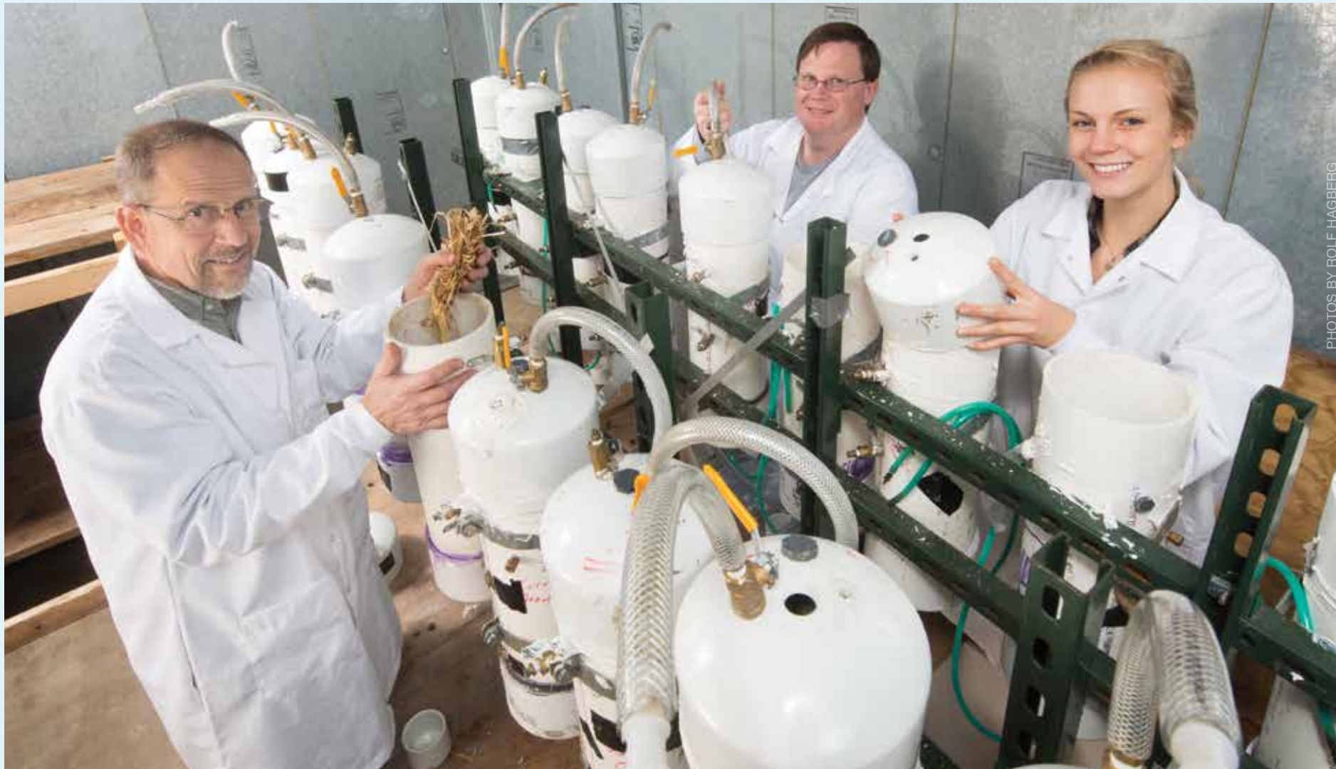
Gary Feyereisen and Todd Schumacher of USDA-ARS work to test agricultural fibers in a denitrifying bioreactor along with Elizabeth Selvik, University of Minnesota student.
