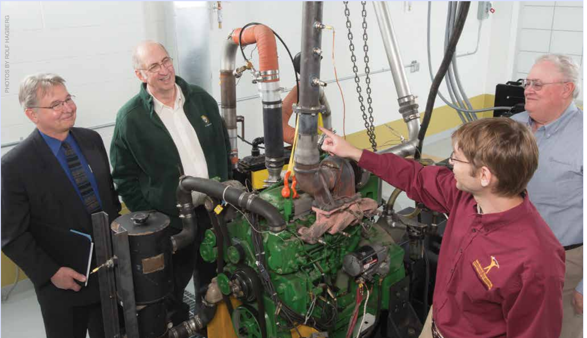
Will Northrop of the University of Minnesota (second from left) shows AURI's Rod Larkins (left) and Minnesota Corn Research & Promotion Council members Richard Peterson (second from left) and Jerry Ploehn (right) how this diesel engine can be retrofitted to use hydrous ethanol, which would decrease the environmental impact of diesel exhaust.
