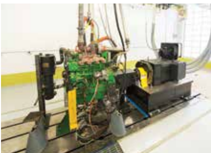
The diesel test engine at the University of Minnesota is being retrofitted to use hydrous ethanol.
