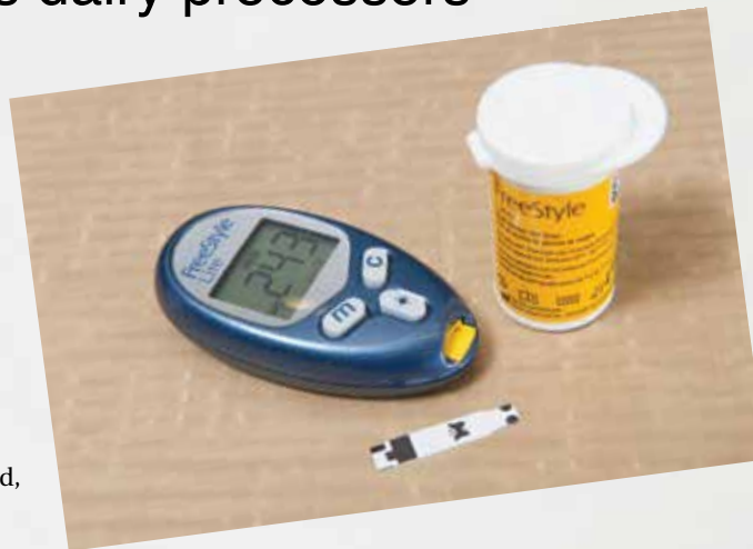
A blood glucose meter can now be used to test the lactose content of milk products.
