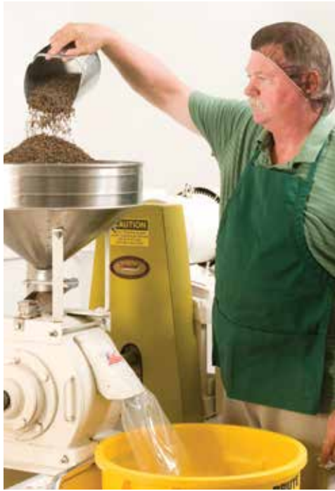
Jay Erckenbrack adds the wild rice to a commercial stone grinder in order to produce quick-cooking stone ground wild rice (polenta) and wild rice flour.
