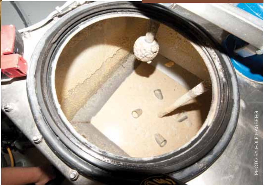
Before fed to swine, ethanol coproducts are mixed in a vat as part of the wet feeding system.
