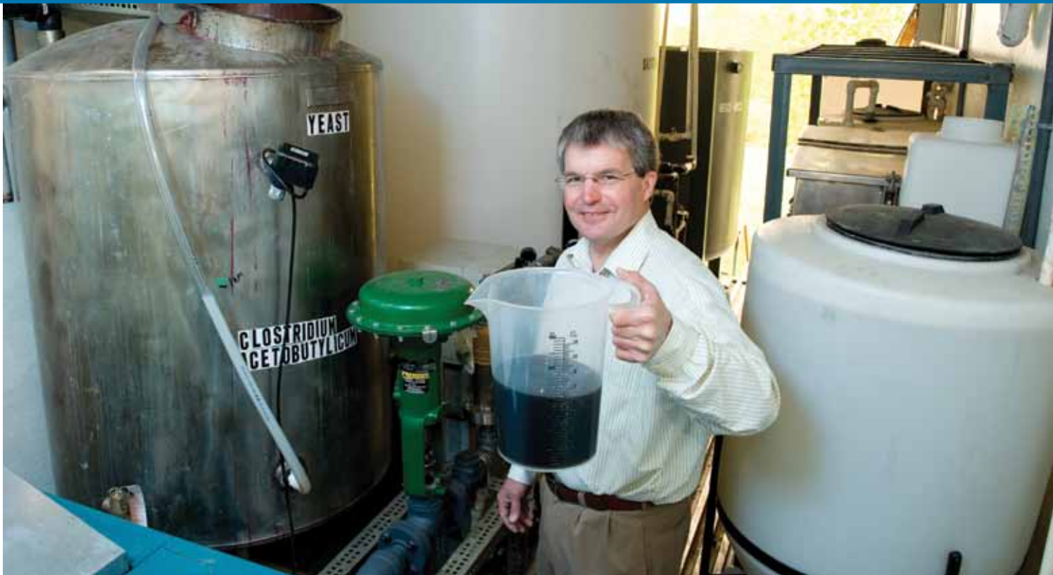
Dave Eid, owner of Encore Bioenergy in Montevideo, holds sorghum “beer” that will be distilled into ethanol in a demonstration plant built in a semi-truck trailer.
