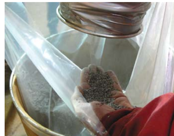
Minnesota biomass-energy plants are producing more than 100,000 tons of ash per year that could have fertilizer value, but the ash has to be granulated before it can be applied to fields. AURI is helping test an ash-densification system, pictured above, where ash enters a processor as a fine powder then exits as granules, which are being tested for the nutrient value in corn test plots.
