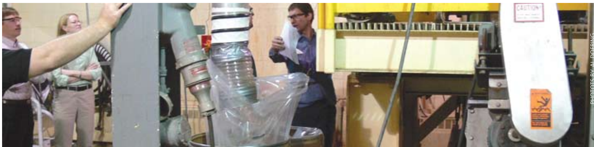
Minnesota biomass-energy plants are producing more than 100,000 tons of ash per year that could have fertilizer value, but the ash has to be granulated before it can be applied to fields. AURI is helping test an ash-densification system, pictured above, where ash enters a processor as a fine powder then exits as granules, which are being tested for the nutrient value in corn test plots.
