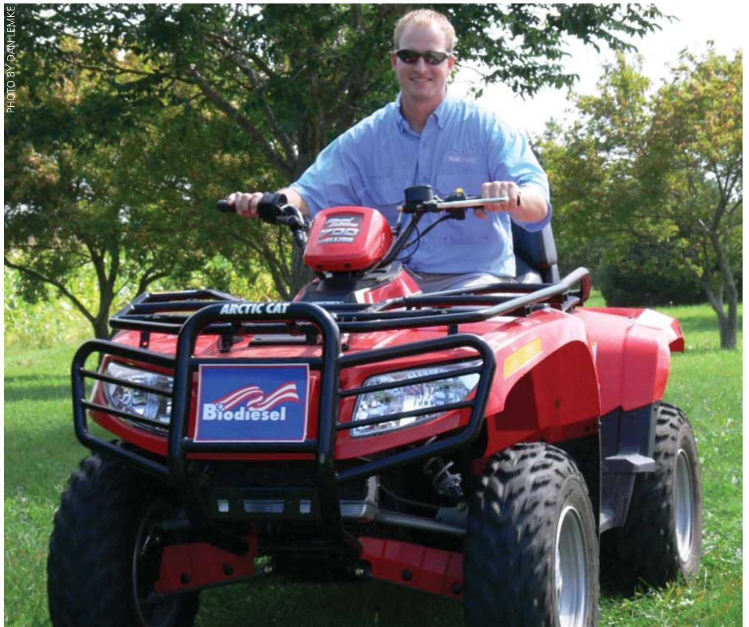
Arctic Cat’s new diesel ATV, test driven by Sam Ziegler of the Minnesota Soybean Grower’s Association runs as well or better on biodiesel than standard fuel, confirmed by tests conducted last winter and this summer. Sponsored in part by AURI’s Center for Producer-Owned Energy, the tests were the first using B20 in small diesel engines.
