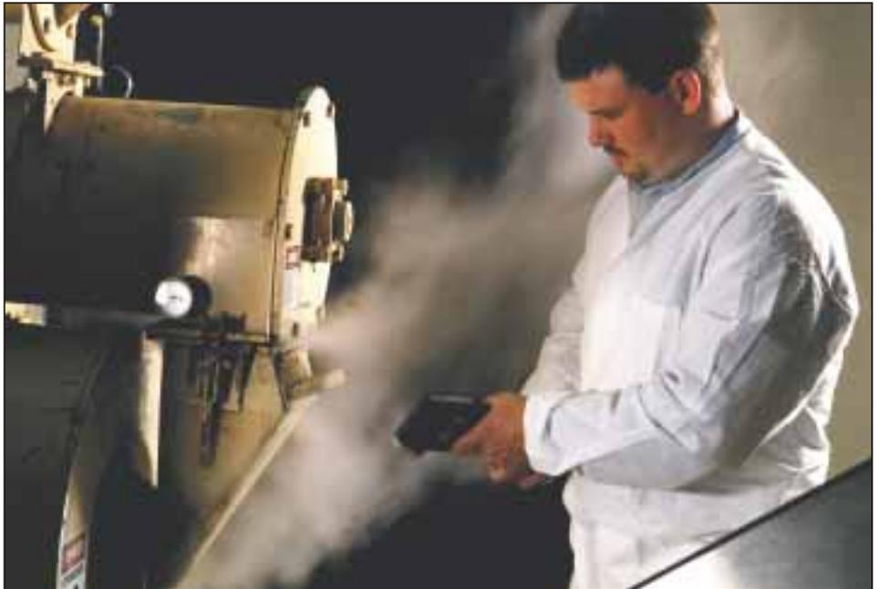
Al Doering uses an infrared gauge to check the temperature of pellets coming out of a mill at AURI's coproducts utilization pilot plant in Waseca. Waste materials such as stems, leaves, hulls, vegetable scraps, and wood fiber are turned into high-value pellets that are burned for energy or used in fertilizers and feeds.
