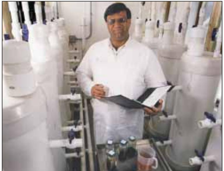
Jack Johnson monitors tanks containing manure gases that have been used to test various ag-based hog odor treatments at AURI's Waseca laboratory.
