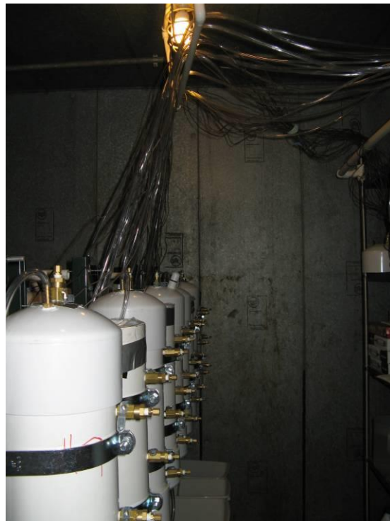
Figure 2. Eighteen bioreactor columns racked and plumbed in a temperature controlled chamber.
