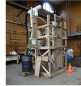
Figure 4: Permeameter in vertical position
