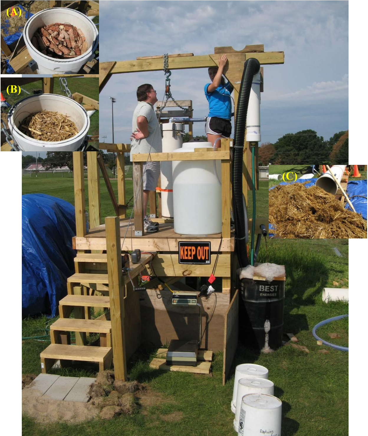
Figure 5. Permeameter built in June and July, 2012, for hydraulic conductivity testing. Insets: Column packed with corn cobs (A) and corn stover (B); column laid horizontally for removal of barley straw (C).
