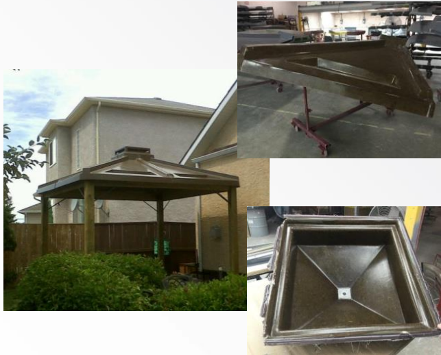
Biocomposite Gazebo Roof Eastside Composites
