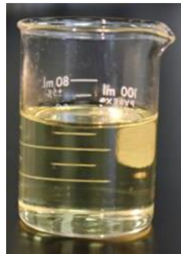
Biodiesel Product (FAME) after Reaction with Methanol in SSC Process, and Removal of Glycol and Water
