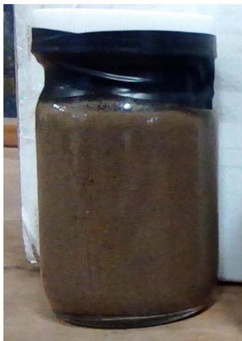
Feed - FOG from WWTP after Debris Removal and Dewatering
