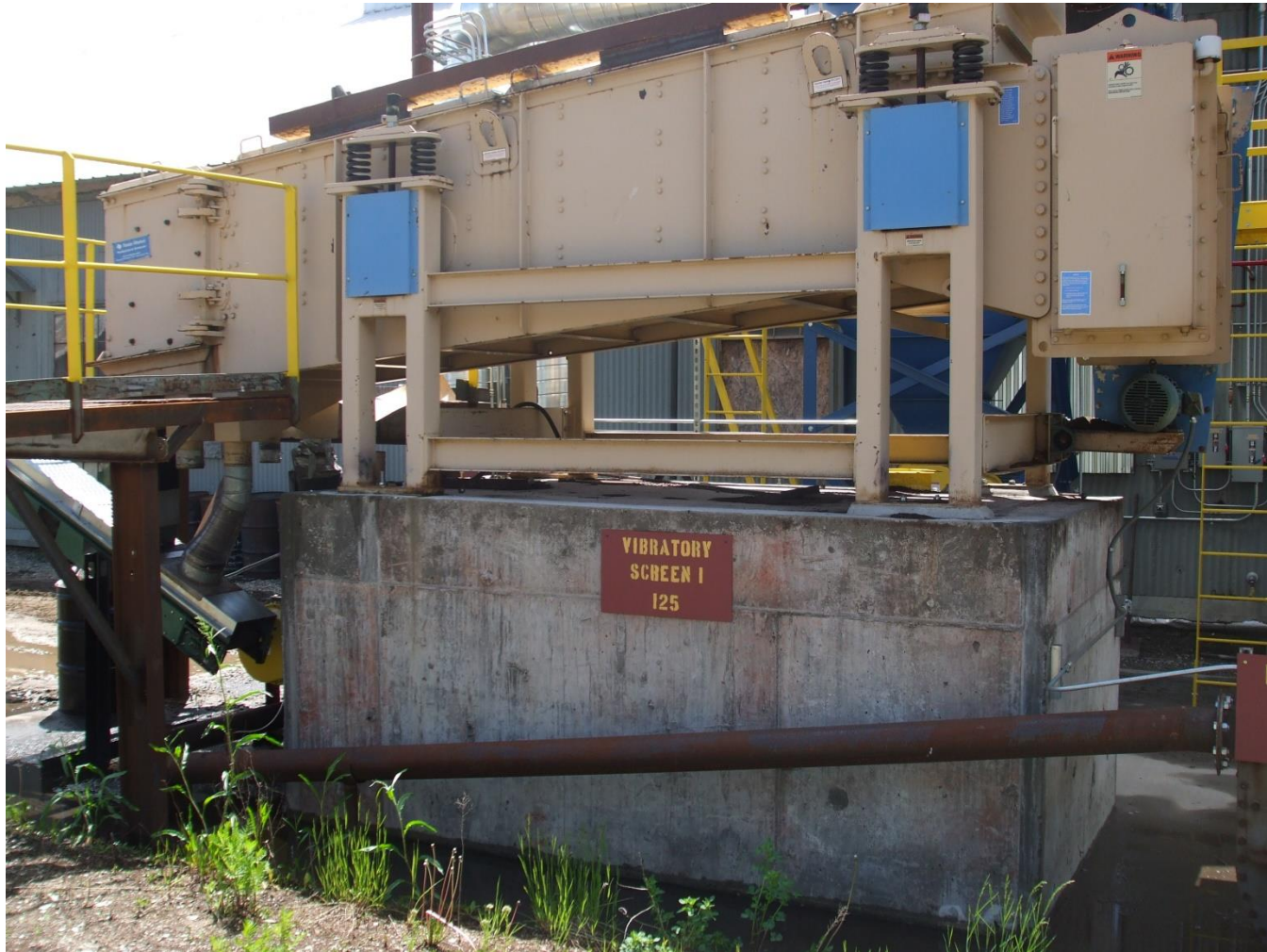
Texas Shaker used to size incoming biomass materials
