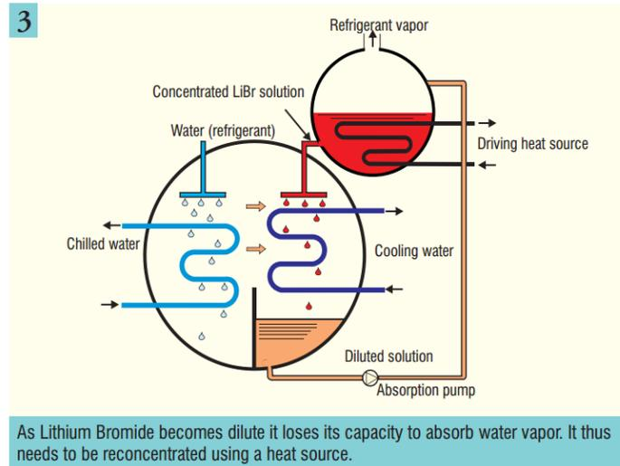
Figure 7. Trane (Thermax) Cooling System – Re-concentrated LiBr
