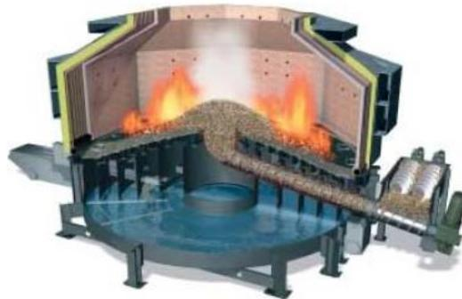
Figure 4. Central Lower Biomass Feed System
