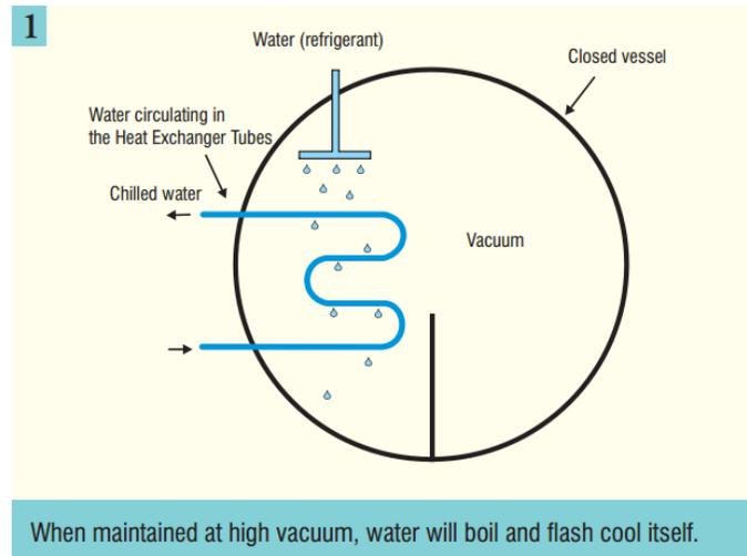
Figure 5. Trane (Thermax) Cooling System – Refrigerating Effect. This diagram illustrates the vaporizing effect of the water refrigerant. Reprinted from <http://www.trane.com/content/dam/Trane/Commercial/global/products-systems/equipment chillers/absorption-liquid/hotwaterdrivenabsorptionchillers.pdf>. Reprinted with permission from Thermax USA.
