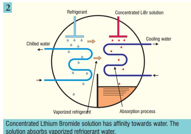
Figure 6. Trane (Thermax) Cooling System – Concentrated LiBr. This diagram illustrates LiBr absorbing the vaporized refrigerant. Reprinted from Trane. (2016). Trane Commercial Heating and Air Conditioning. Trane University. Retrieved from <http://www.trane.com/commercial/north-america/us/en.html>. Reprinted with permission from Thermax USA.
