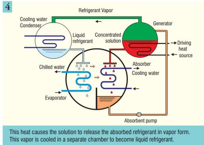
Figure 8. Trane (Thermax) Cooling System – Liquid Refrigerant
