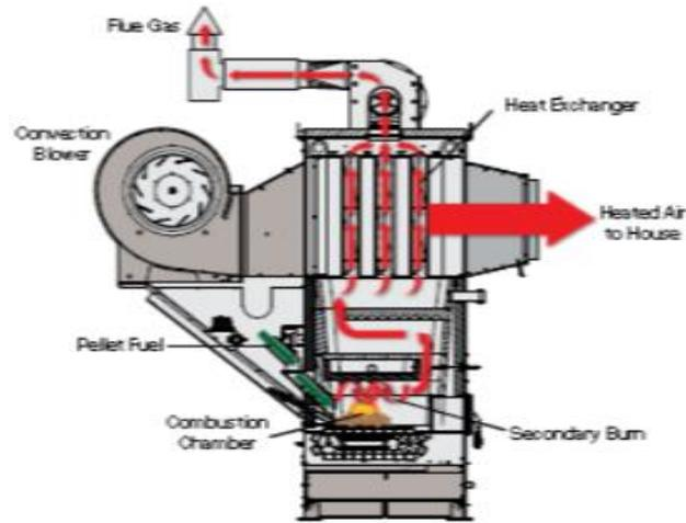
Figure 3. Biomass Furnace Diagram
