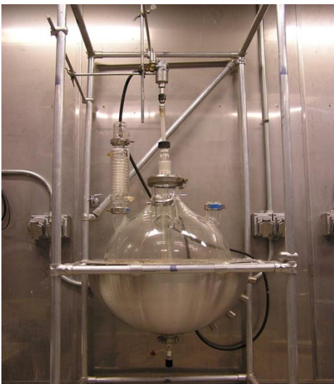
Picture 3. Apparatus for ethanol extract – micelle processing (ethanol removing, oil separation from solubles).
