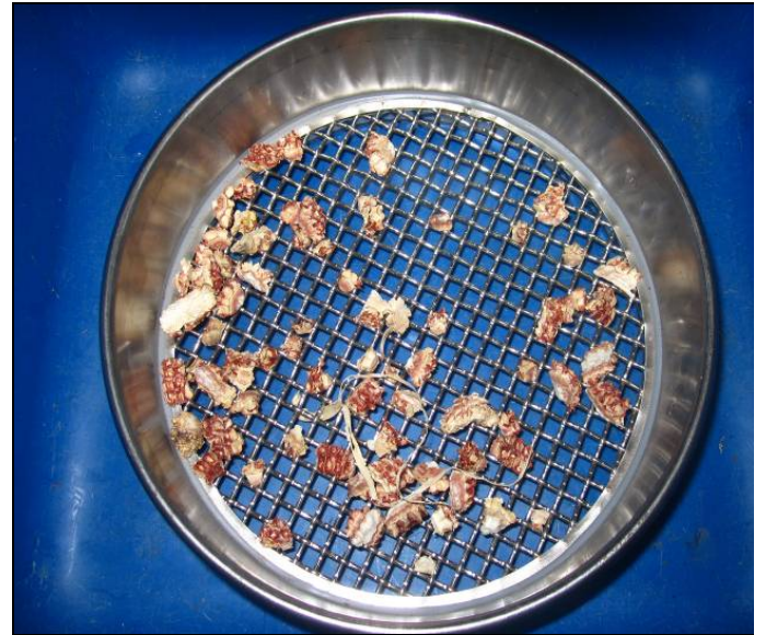
Corncoobs retained on 6.3 mm sieve
