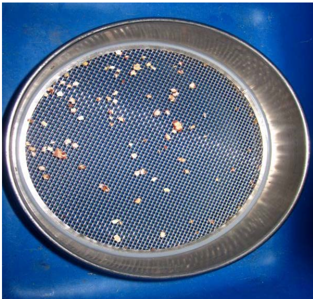
Corncoobs retained on 2mm sieve
