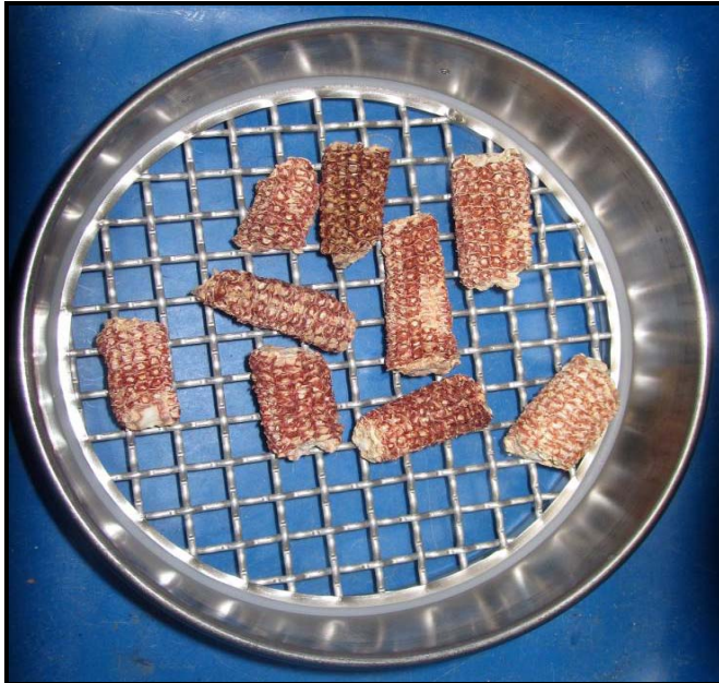
Corncoobs retained on 12.5 mm sieve
