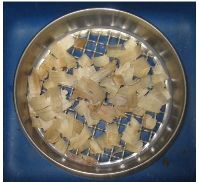
Tamarack shavings retained on 12.5 mm sieve
