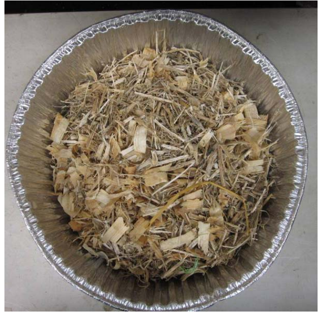
Jack Pine and Soybean straw mixture
