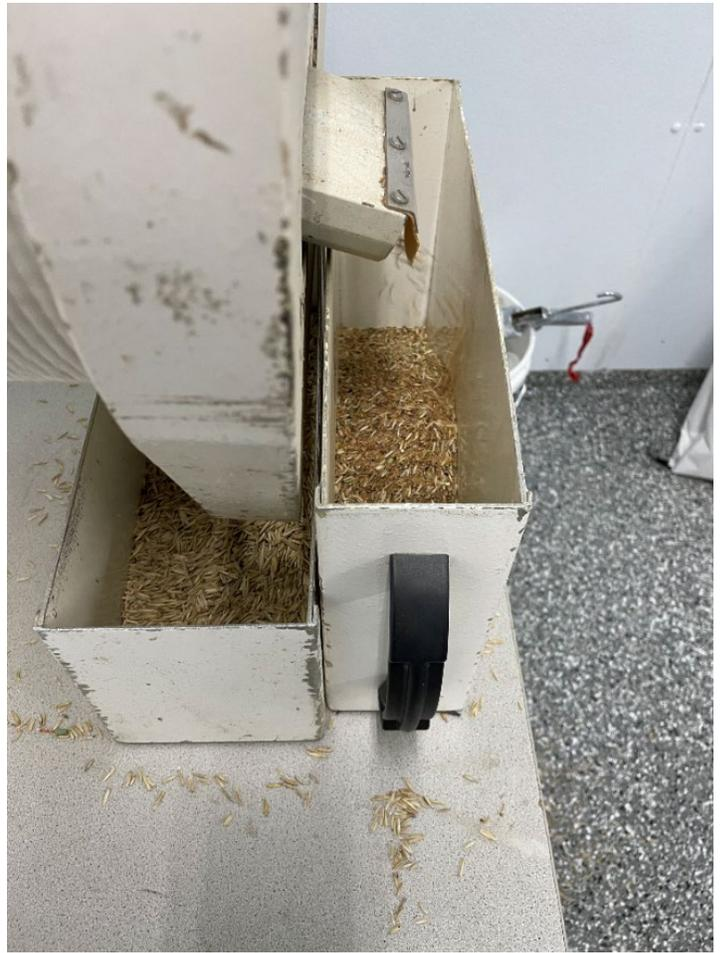
Figure 15. Cleaned Dehulled (right) and In-hull (left) Kernza® after indent separation. (Center) shows adjustable arm to alter grain cuts
