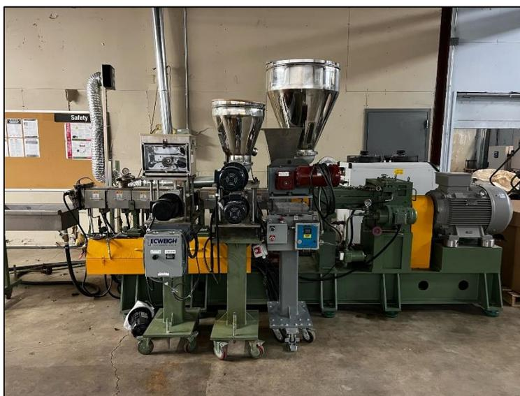
**Figure 1.** 43mm Nanjing Giant Twin Screw Extruder
