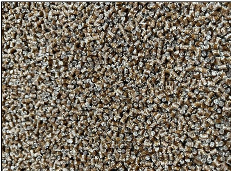
**Figure 2.** PLA/Kernza Biocomposite Pellets for Injection Molding
