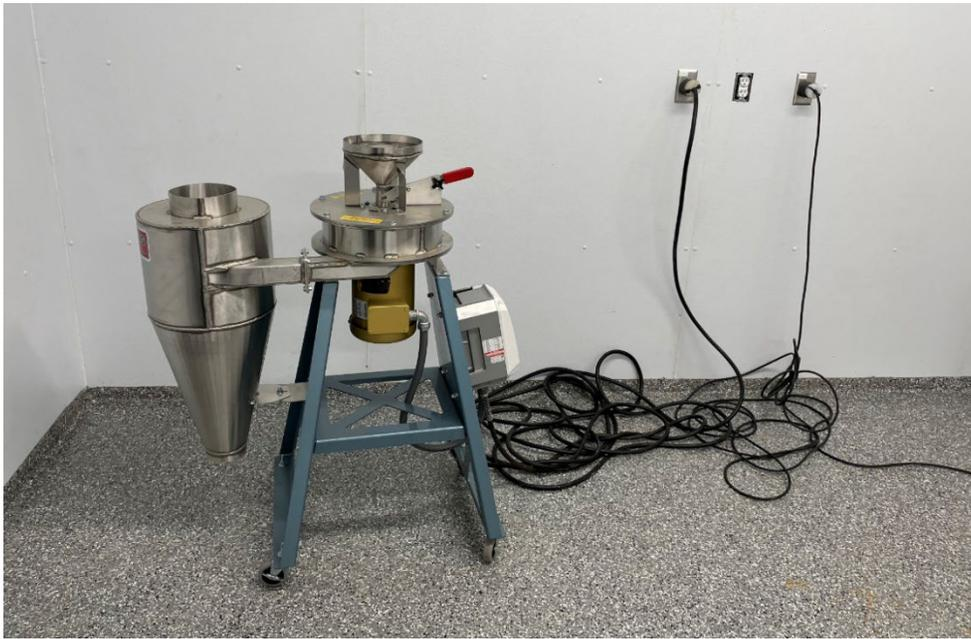
**Figure 14. Impact Separator 'in-action' producing in-hull grain for malting**
